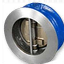
Two semi-circular plates are mounted to the valve body by hinge pin. When the fluid flows, each plate opens in a V shape centering on the hinge pin and fully opens up to the stop pin.
